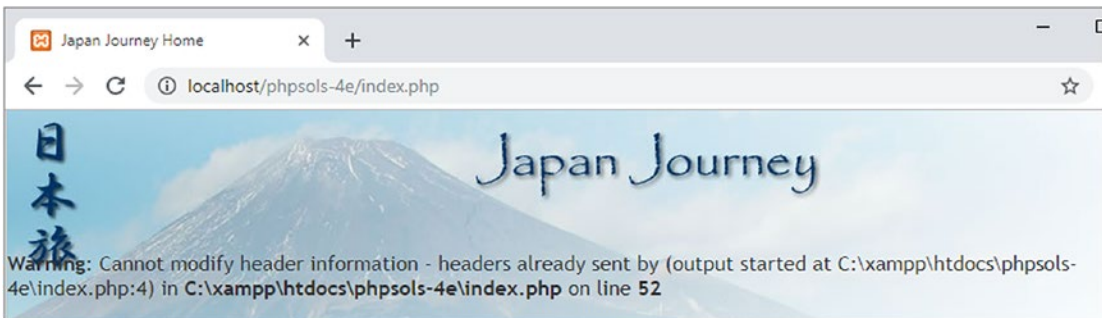
Figure 5-15. The header() function won't work if output has already been sent to the browser
